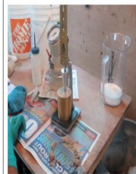
Photo 09: Vicat cone penetration test performed on fresh mortar sample.
