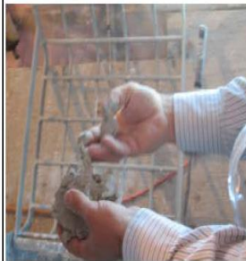
Photo 08: Mortar is of the good consistency and sticks to the fingers.
