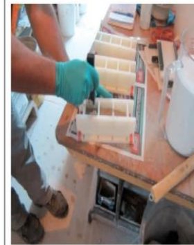
Photo 11: Cubes of fresh mortar taken for compressive tests.
