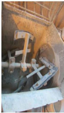
Photo 02: New paddles were installed, which are now reaching the sides of the bucket.
