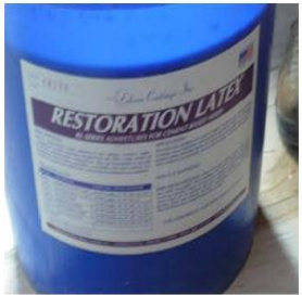
Photo 03: Polymer used for mortar: restoration latex RL1 by Edison Coating Inc.
