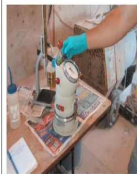
Photo 10: Air content test performed on site on fresh mortar sample.
