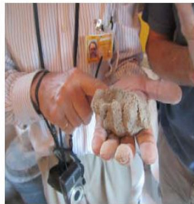
Photo 07: Mortar is too dry and doesn't stick to the fingers.
