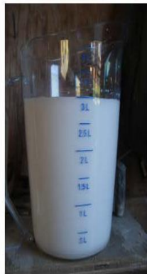
Photo 05: Liquid composed of 50% restoration latex RL1 by Edison Coating Inc. and 50% potable water is to be carefully mixed separately before being added to the dry mortar mix.
