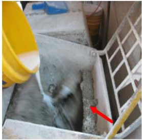
Photo 01: Mixer's paddles not reaching the sides of the bucket, creating a crust of dry ingredients on the sides of the bucket.
